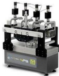
Four Point Bending Apparatus (Pneumatic)
